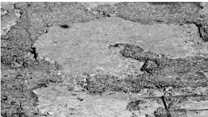
◀ Wire reinforcing mesh placed close to surface. Corrosion of the reinforcing steel causes the surface mortar to spall. Very difficult to patch and repair.
