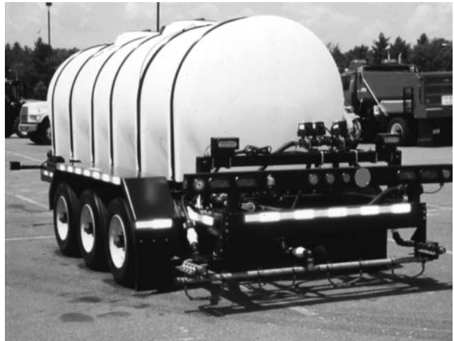
Often anti-icing programs start small with tanks on the back of a patrol truck LEFT. A large tanker RIGHT is more efficient for anti-icing a larger road system.
