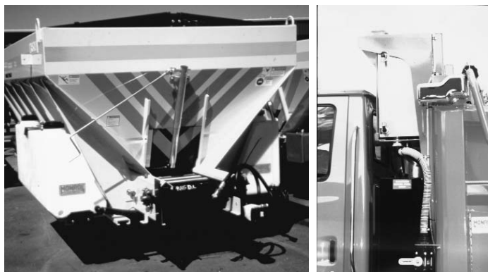
Tanks for pre-wetting liquid: saddle-bags on a hopper spreader LEFT, and at the front of a dump body with a tailgate spreader RIGHT.
