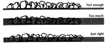
When properly applied, asphalt covers two-thirds of the aggregate.
